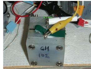
Figure 2: Microbial fuel cell, attached to the voltmeter
