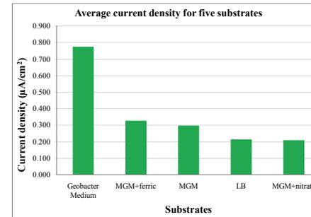
Figure 5: Average current density produced by each of the five substrates
