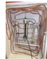
Fig. 4 Uncovered column inside the temperature controlled chamber, with control panel and peristaltic pump
