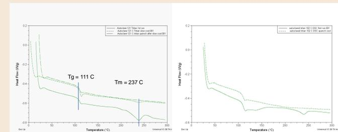
Heat Flow vs. Temperature Graphs for Tritan™ Copolyester Bottles Autoclaved at 121°C
