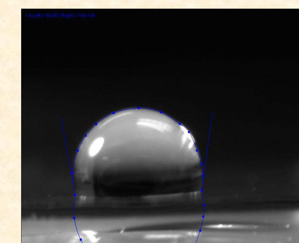
Figure III-2: Analysis of a water droplet on an OTS-coated glass disc using Drop Analysis Package for ImageJ. Contact angle: 99.9°.
