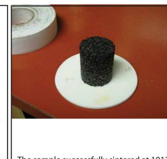
The sample successfully sintered at 1012 °C for one hour. The cylinder is a 1.125" diameter and 1.2" height.
