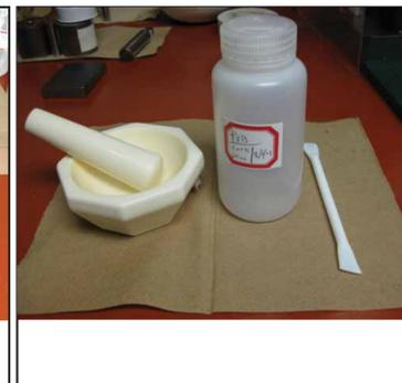
The mortar, pestle and plastic stirrer are used to mix both the Kalapana basalt sand with the PVB, a binder also known as polyvinyl butyral. A 5 wt % solution of PVB was used to bind the sand.
