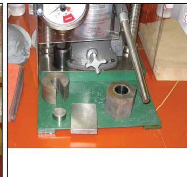
The tools here are used to make the sample its size and shape. The press is done manually and requires applying 16,000 lbs to create a sample. The sample is shown below.
