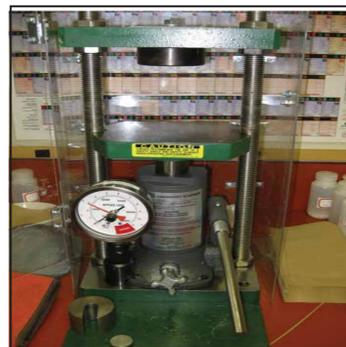
This is the press that is used to consolidate the Kalapana basalt glass before it is sintered.
