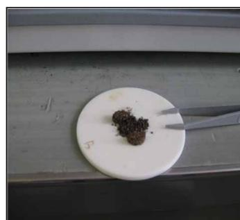
The test sintering temperature started at 500 °C and went up to 1020 °C. At 1000 °C is when the sand begin to sinter, but at 1020 °C is when it is more stable.
