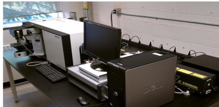
Set up of Raman Spectrometer
