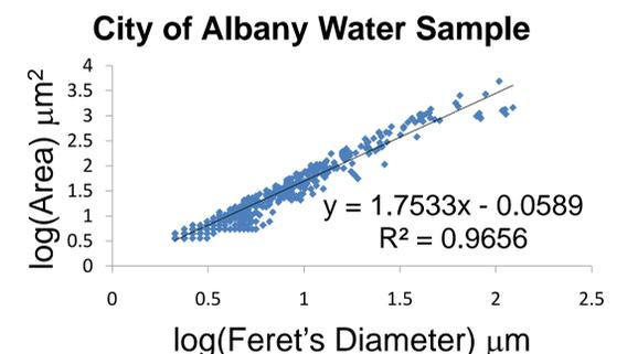
**Figure 4:** Graph of particles showing fractal dimension patterns from water for a City of Albany project analyzing river water samples. The particles are non-Euclidean with a  $D_2$  fractal dimension of 1.75
