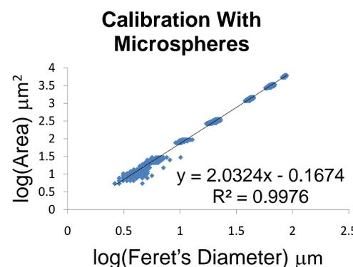
**Figure 4:** Calibration run of latex microspheres of varying sizes to show that they follow Euclidean geometry (i.e., slope =  $D_2 = 2$ ).
