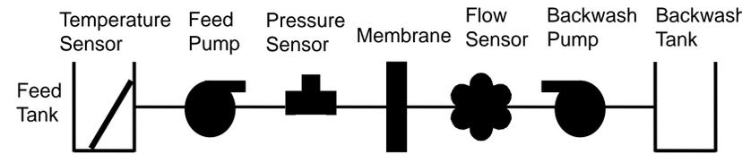
**Figure 2:** Schematic of the basic components in filtration system
