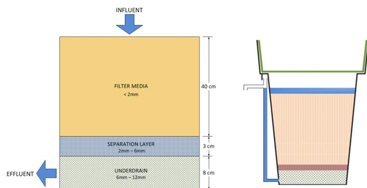
**Figure 1:** Biosand Filter Structure.
