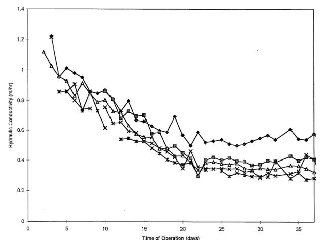
**Figure 2:** Decreasing hydraulic conductivity with operation time. (Buzunis, 1995)
