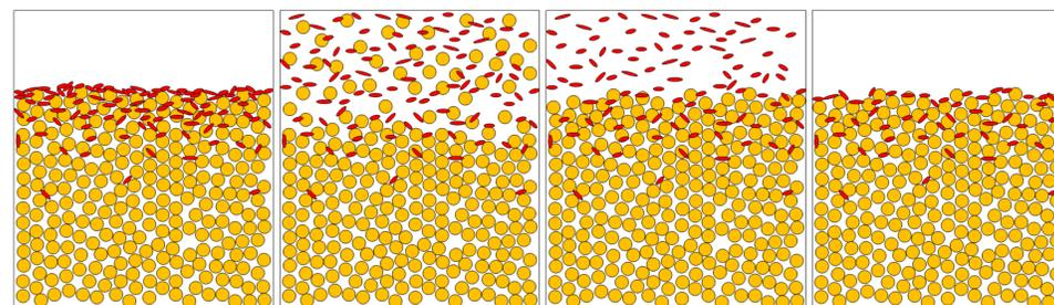
**Figure 3:** Biosand Filter agitation process.
