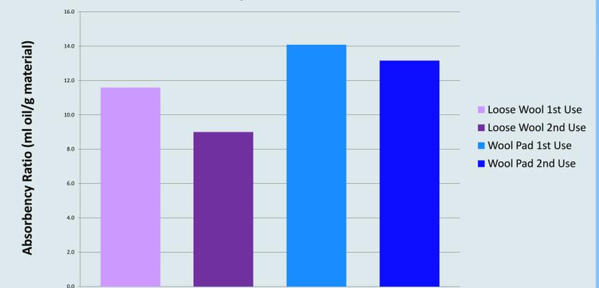
Figure 2. Data obtained with triplicate trials of crude oil absorbed by various forms of wool. The nonwoven wool blanket has the highest absorbency ratio.
