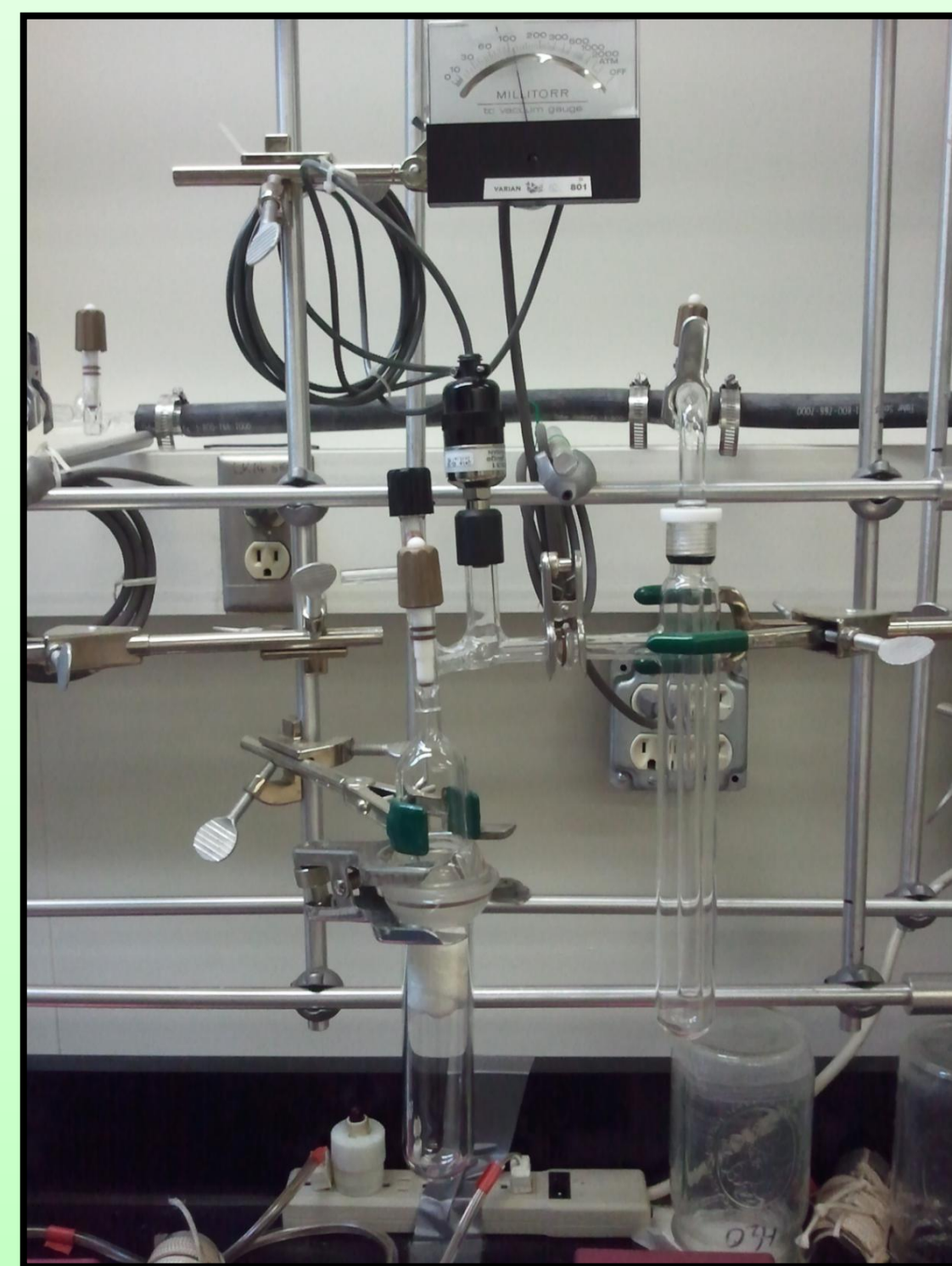
Image 1. Section of glass line used for water extraction. Displayed are the sample holder (on left with glass wool) and water collection tube (on right)
