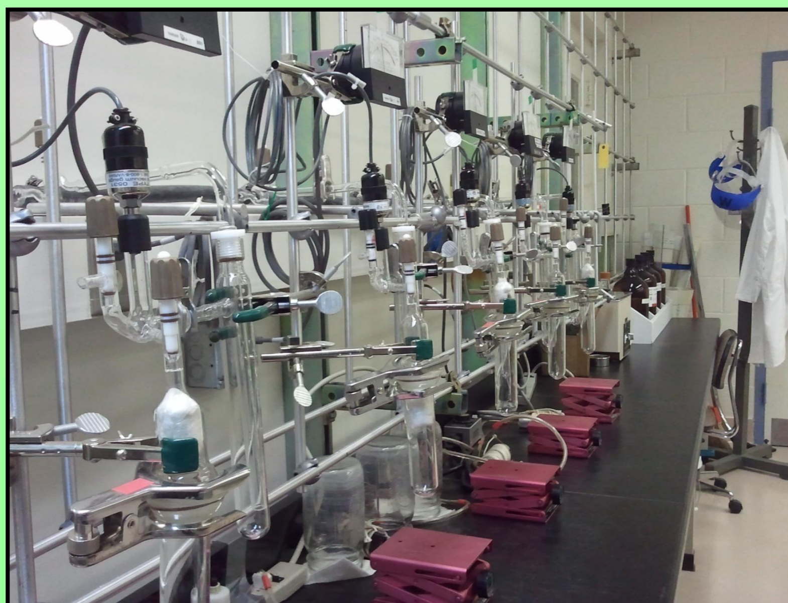
Image 2. Section of glass line showing five stations used for water extraction
