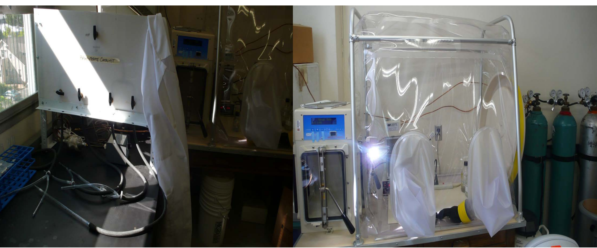
Fig. 5 : Culturing is done under anaerobic conditions by sparging the media and samples under nitrogen gas for 15 minutes in the gassing station on the left. Inoculation occurs in the glovebox on the right.
