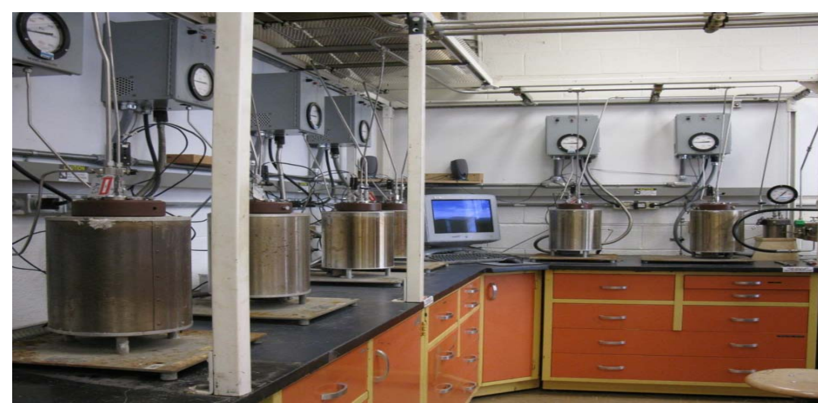
Fig. 6: Autoclaves in which the samples were incubated in at 35°C and 1200 psi.
