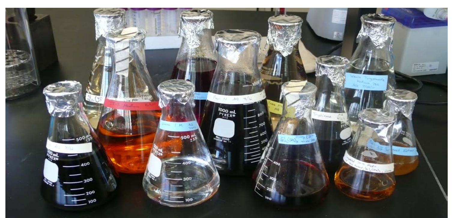
Fig. 4: The media and components of media shown here are Magot's N,M, and Acidophilium media for iron reducers. (Basso, 2009) Postgate's B and C media for sulfate reducers. (Geomicrohandbook citation) No hydrogen utilizing media were selected.
